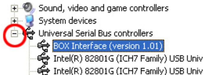
3. Highlight the “BOX Interface (version x.xx)” (or “USB Plus interface) and select “uninstall” on the top menu bar. This will uninstall all associated drivers for the interface.
